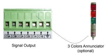
There are three section controllers, (C1A, C1B), (C2A, C2B), (C3A, C3B), each of them has two wire connectors. They work respectively.
