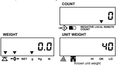
Press **U.WT** key to complete sampling operation & enter into counting mode.
