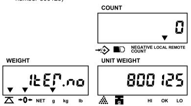
5. Enter item name by using ASCII code. Note that you can enter up to 16 digits. Refer to ASCII code on P18.
