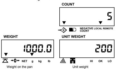
Press TOTAL key to enter into accumulation status mode. At this moment, total accumulated weight is shown in WEIGHT window, total accumulation times is shown in UNIT WEIGHT window and COUNT window displays accumulated count.
