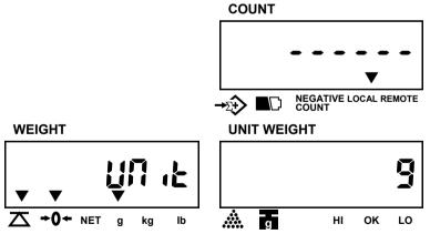
Press **ENTER** key for determination and enter into calibration mode.
