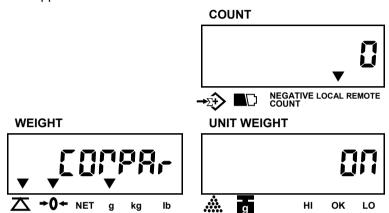
2. Press **MOVE** key to revolve the system-preset three section control signal.(on, off)
