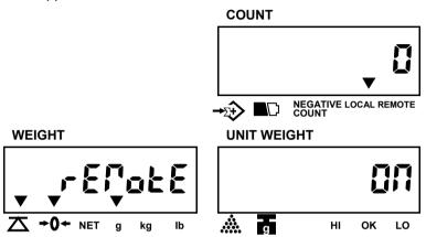
2. Press **MOVE** key to revolve the system-preset remote platform(on, off).
