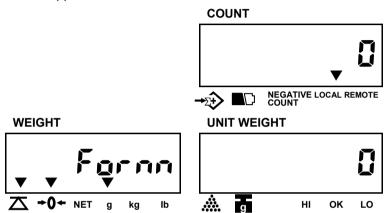
Press MOVE key to revolve the system-preset file name of the format. (Default setting: 0)
