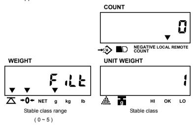
2. Press **MOVE** key to revolve the system-preset stable class range. The smaller number selected, the shorter time for display stability (0=off, 1=0.05d, 2=0.15d, 3=0.25d, 4=0.35d, 5=0.45d).
