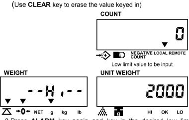
3. Press ALARM key again and key in the desired low limit
