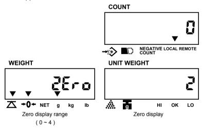
2. Press **MOVE** key to revolve the system-preset zero display range (0=off, 1=0.5d, 2=1d, 3=2d, 4=3d).
