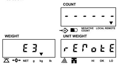
While when the local platform is not connected well, the display will show:
