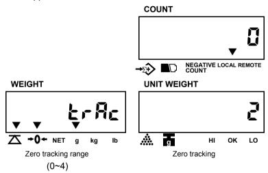
2. Press **MOVE** key to revolve the system-preset zero tracking range.
