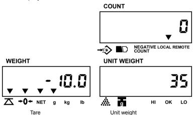
Place the sample on the pan, weight window shows the net weight.
