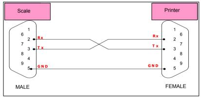
Connect EC-II and Printer using same cable. [male(EC-II) – female(DLP-50)]
