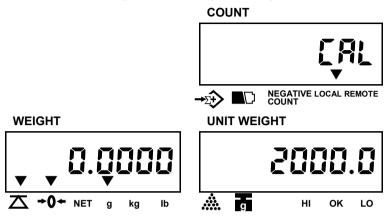
4. Put a weight on the pan same as what exactly shown in the UNIT WEIGHT window, then press the ENTER key to confirm the operation.
