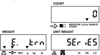
2. Press **MOVE** key to revolve the system-preset the transmit method of extra display.(5£86£. 5£6.65)
