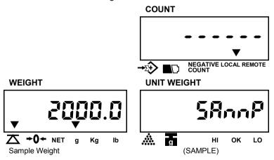
4. The sampling operation is completed while stable display appears as below :
