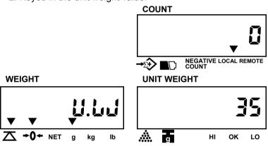
If sample operation is done before entering this mode, unit weight window will automatically show the unit weight.
