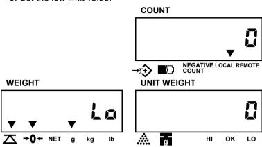
10. Enter a address cell (1~200, total 200 cells available) by pressing any of the numeric keys (0~9), then press the ENTER key to store the above information into the address cell.
