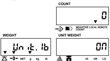
Press MOVE key to revolve the system-preset units of measure ( ON, OFF ).
