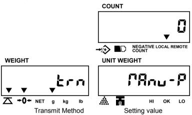
Press MOVE key to revolve the system-preset transmit method.
