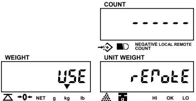
3seconds later, the scale returns to normal mode and **REMOTE** indicator will be on. Remote platform is used.
