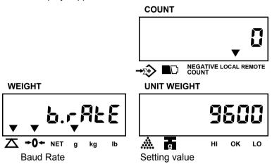
Pess MOVE key to revolve the system-preset baud rate.(2400, 4800, 9600)
