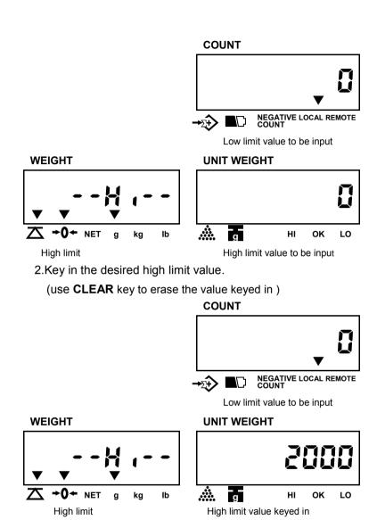
3.Press ALARM key again and key in the desired low limit value as indicated below. (Low limit value effective only after high limit is preset)
