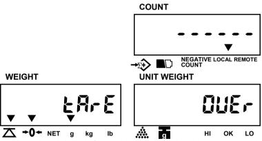
When the high limit for weight is larger than the max.capacity, the display will show:
